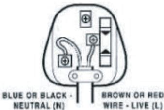
The BLUE wire must be connected to the terminal marked with the letter N
