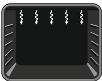
**Grilling function:** Switch on the GRILL function using the top oven function control knob. The oven thermostat and warning lights will illuminate, and the grill heating element will switch on. The
