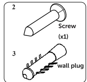
The document bag contains an anti-tilting kit. Loosely attach the anti-tilting bracket (1) to the wall using the screw (2) and wall plug (3), following the measurements shown in the figure and table below. Adjust the height of the anti-tilting bracket so that it lines up with the slot on the cooker and tighten the screw. Push the appliance towards the wall making sure that the anti-tilting bracket is inserted into the slot on the rear of the appliance.
