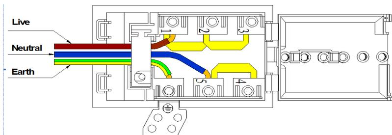
**Warning:** Connect the power cord must be in accordance with the instructions listed in the table below
