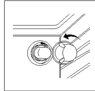
Replace the glass cover. Reconnect the appliance to the mains power supply.
