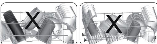
Incorrect loading can cause poor washing and drying performance. Please follow the manufacturer's recommendations for a good performance result.
