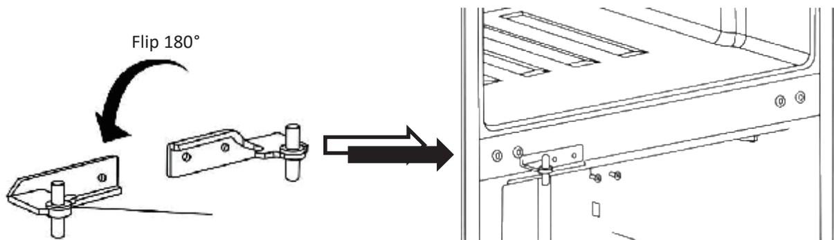
6. Remove the hinge stopper from the bottom of the fridge door and fix the spare hinge stopper that is supplied as an accessory (packaged with the IB) to the opposite side of the fridge door, ensuring it is fixed securely.
