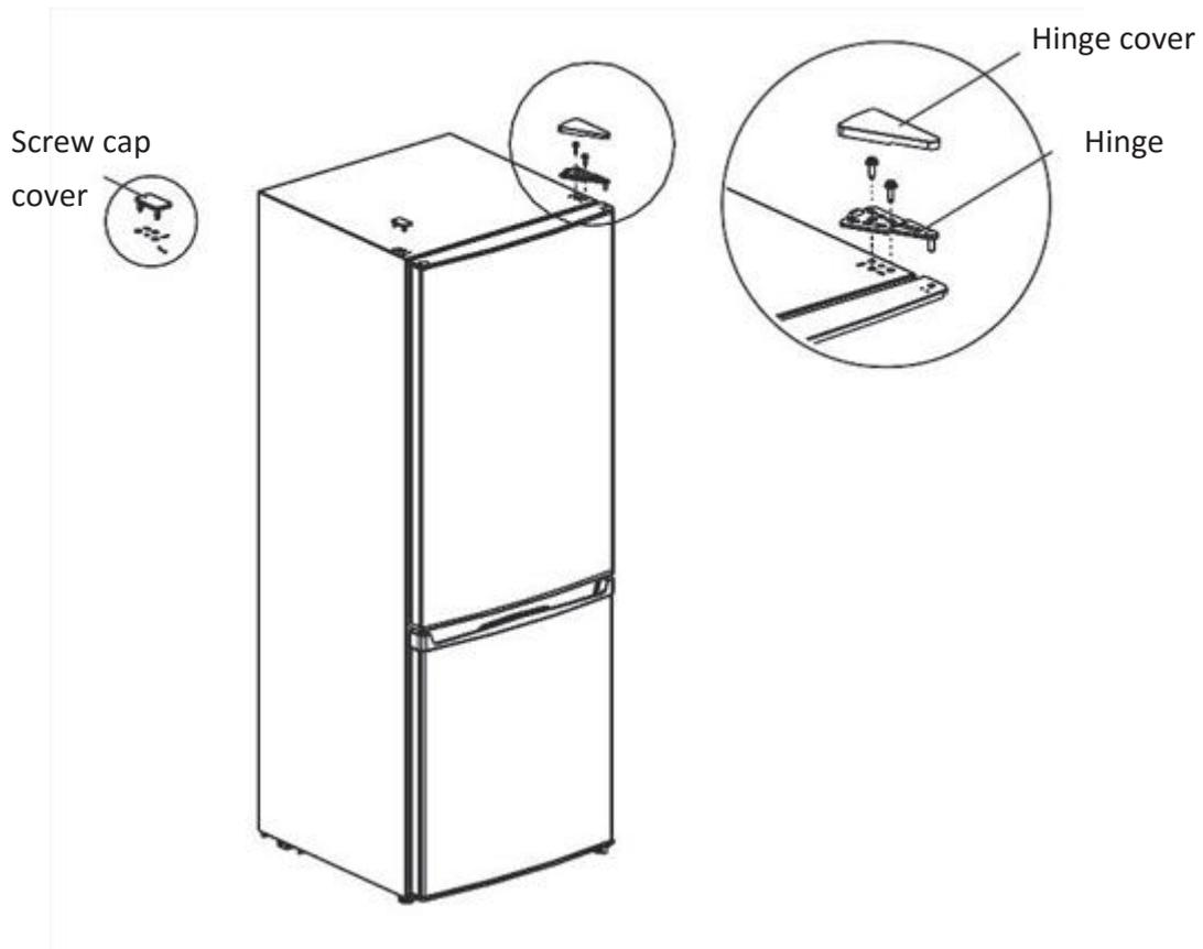
2. Remove the screw cap covers that are on the top left of the unit and fix them on to the opposite side.
