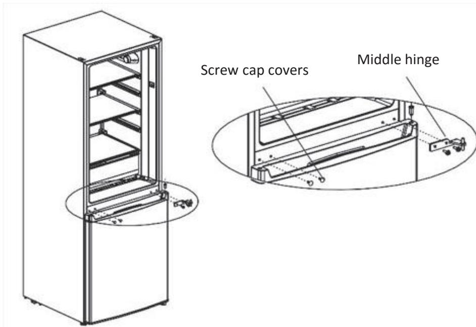
4. Remove the hinge plug from the top of freezer door and fix it to the opposite side. Then remove hinge stopper from the bottom of the freezer door and fix it to the opposite side, ensuring it is fixed securely. Tilt the appliance carefully, no more 45 degrees and remove the adjustable foot. Take off the bottom hinge by removing the screws. Reattach the hinge to the left side of the appliance, reinstall the adjustable feet and place the freezer door back on.
