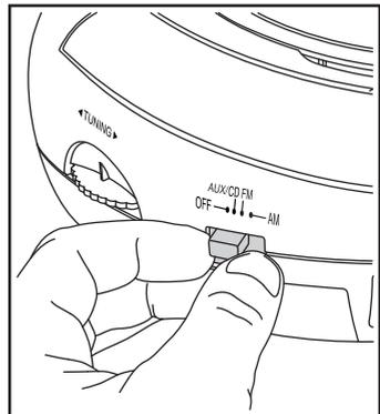
Tune the radio by turning the TUNING dial on the side of the CD Boombox to the correct frequency.
