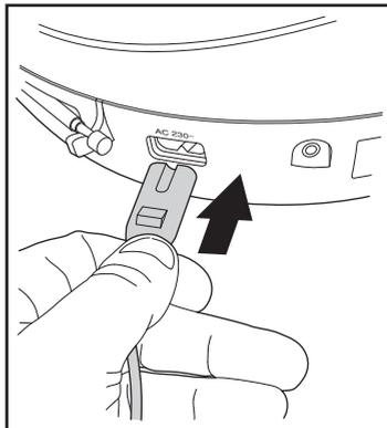
Insert the plug on the other end of the power cord into a mains socket and turn the power on if needed.
