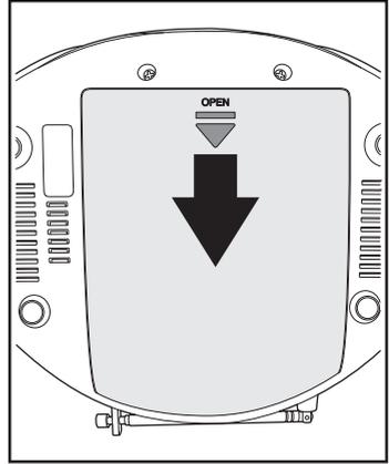
Insert the eight type C batteries following the directions in the bottom of the battery compartment.
